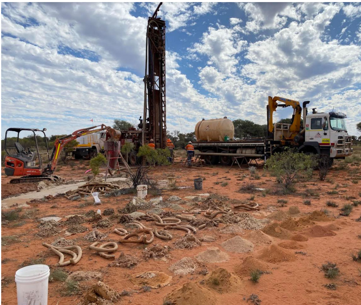
Figure 11. Water Well rig drilling at LWP002.
