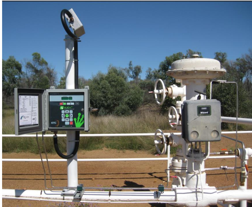
Kincora #40 well site intermitter unit – installed Nov 2022
