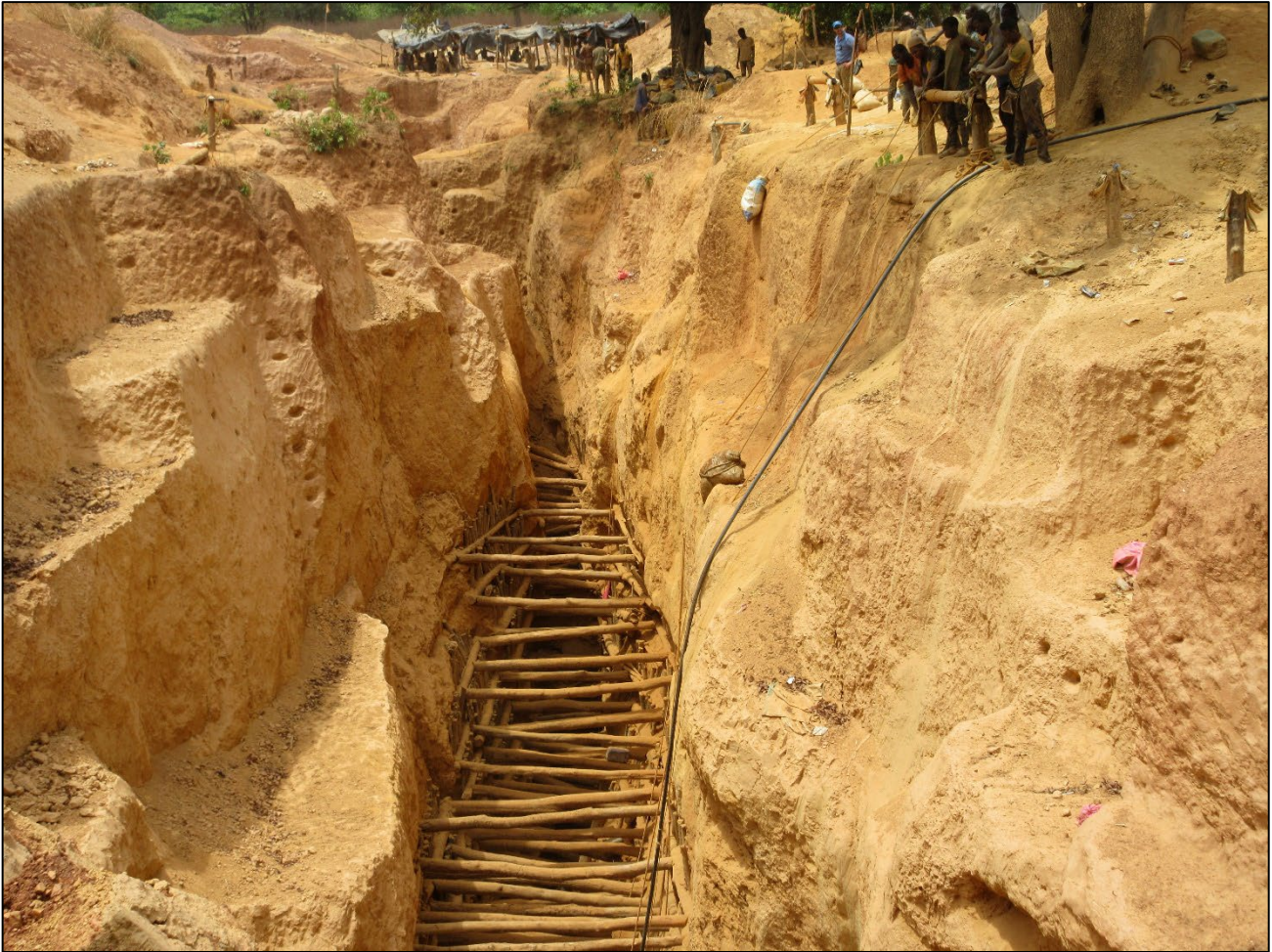
Figure 5: Artisanal mining site on large quartz NW vein at Tchaga North - photo location on Figure 4
