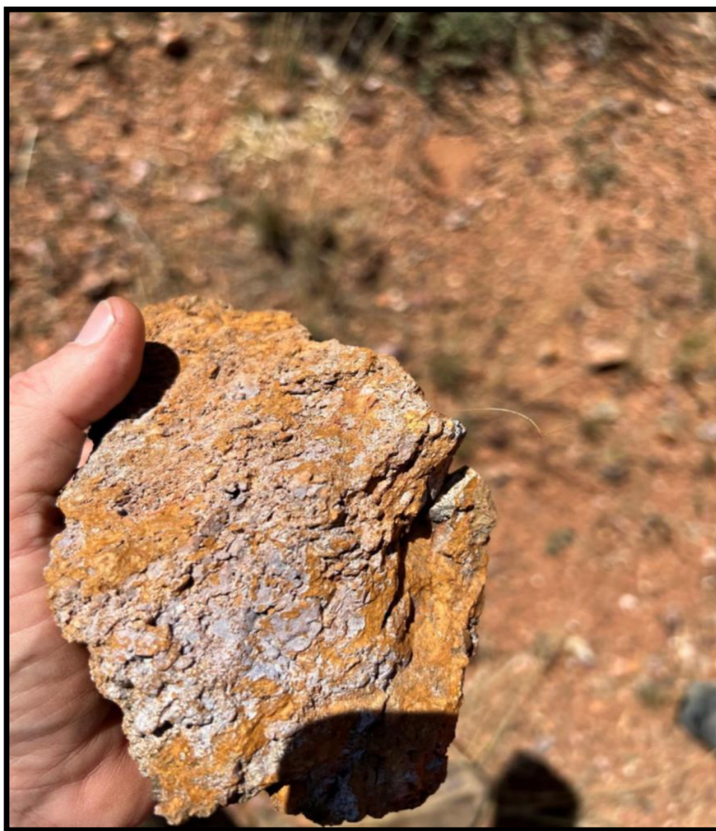
Figure 4. Hand Specimen; Sample T23-007 (3.38% TREO)
