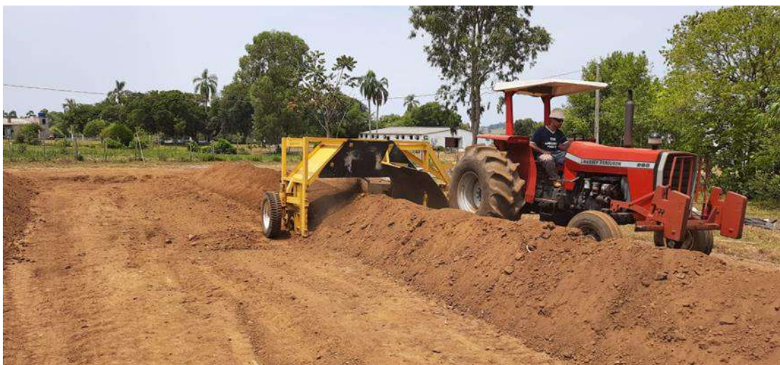
Figure 17: Prototype of windrow turner in operation
