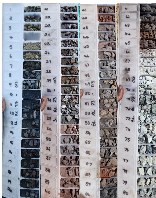
Figure 3. Chip tray photographs from hole SLRC23-013. The image shows a 60m interval of graphite mineralisation from 6m to 66m downhole. True thickness in unknown.
