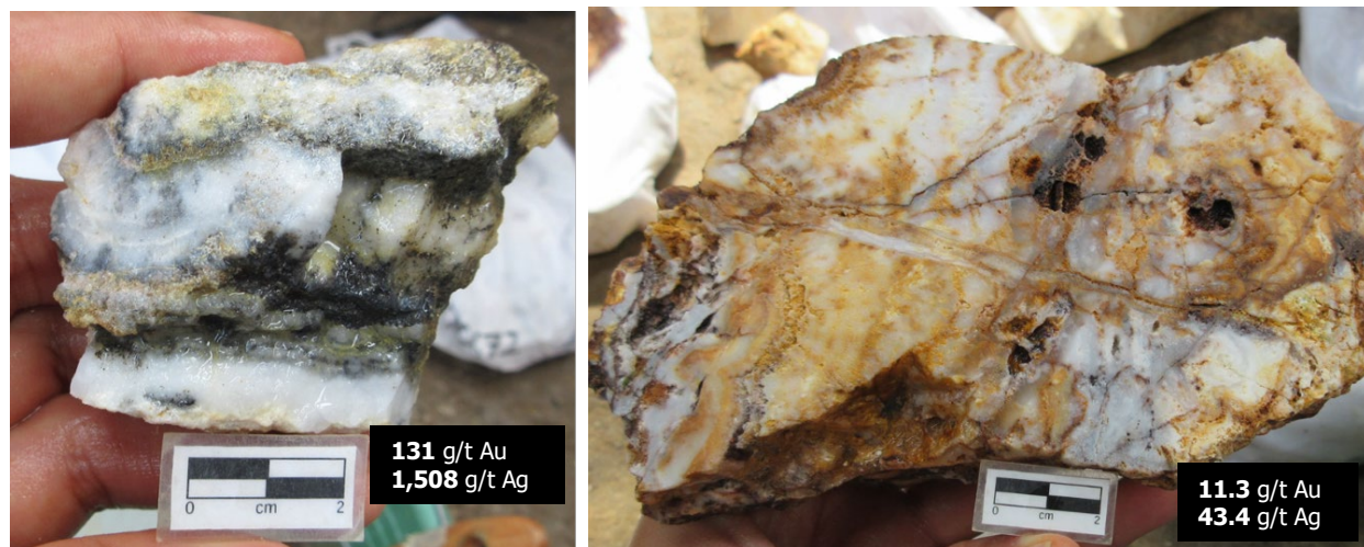
Figure 2: Photos of samples of vein material taken from artisanal miner pits. Refer to Figure one for sample locations. Both samples show the presence of crustiform banded quartz with thin dark-grey ginguero bands.
