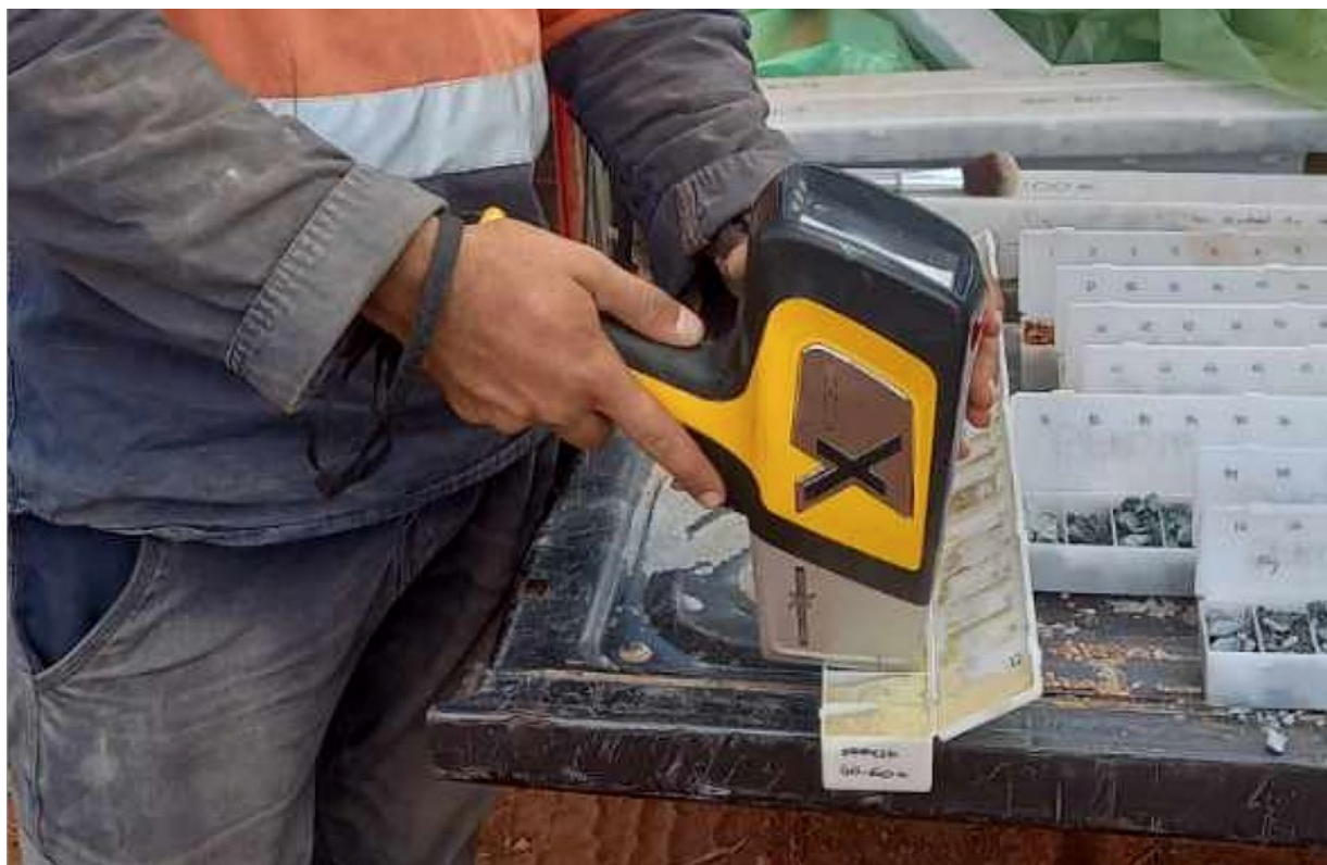
Figure 3: The hand-held XRF gun being used at the drill site to test nickel levels and to select samples for assays
