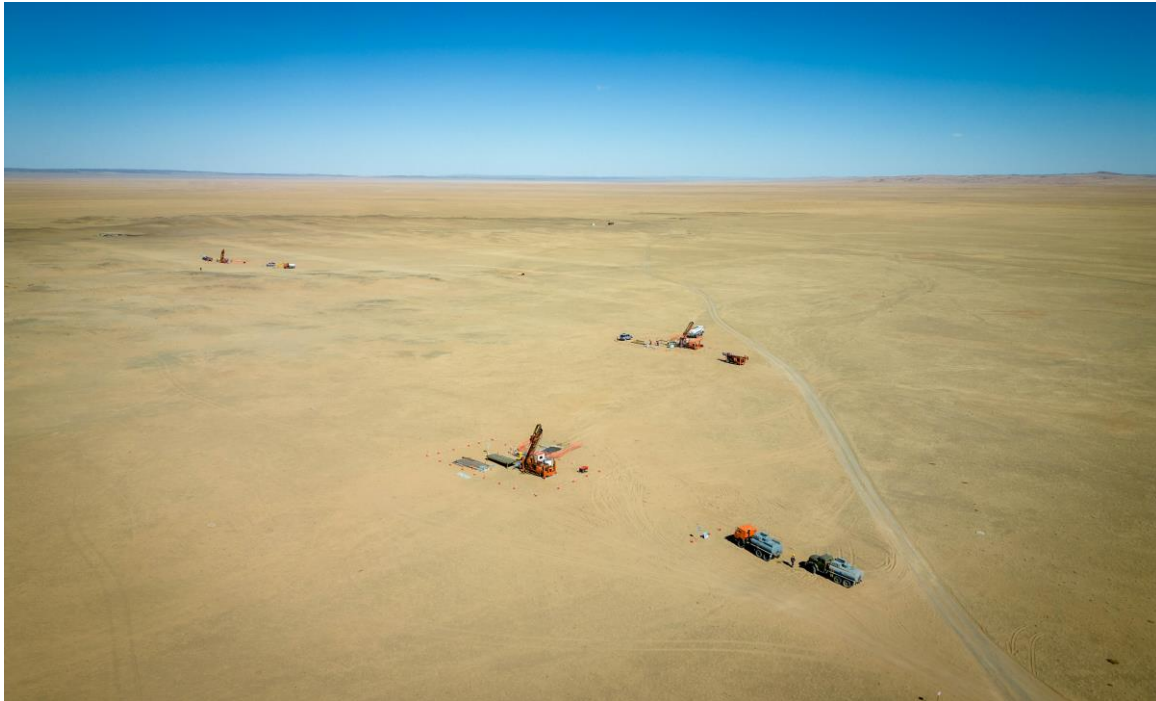
Figure 2: Three diamond drill rigs drilling at Stockwork Hill.
