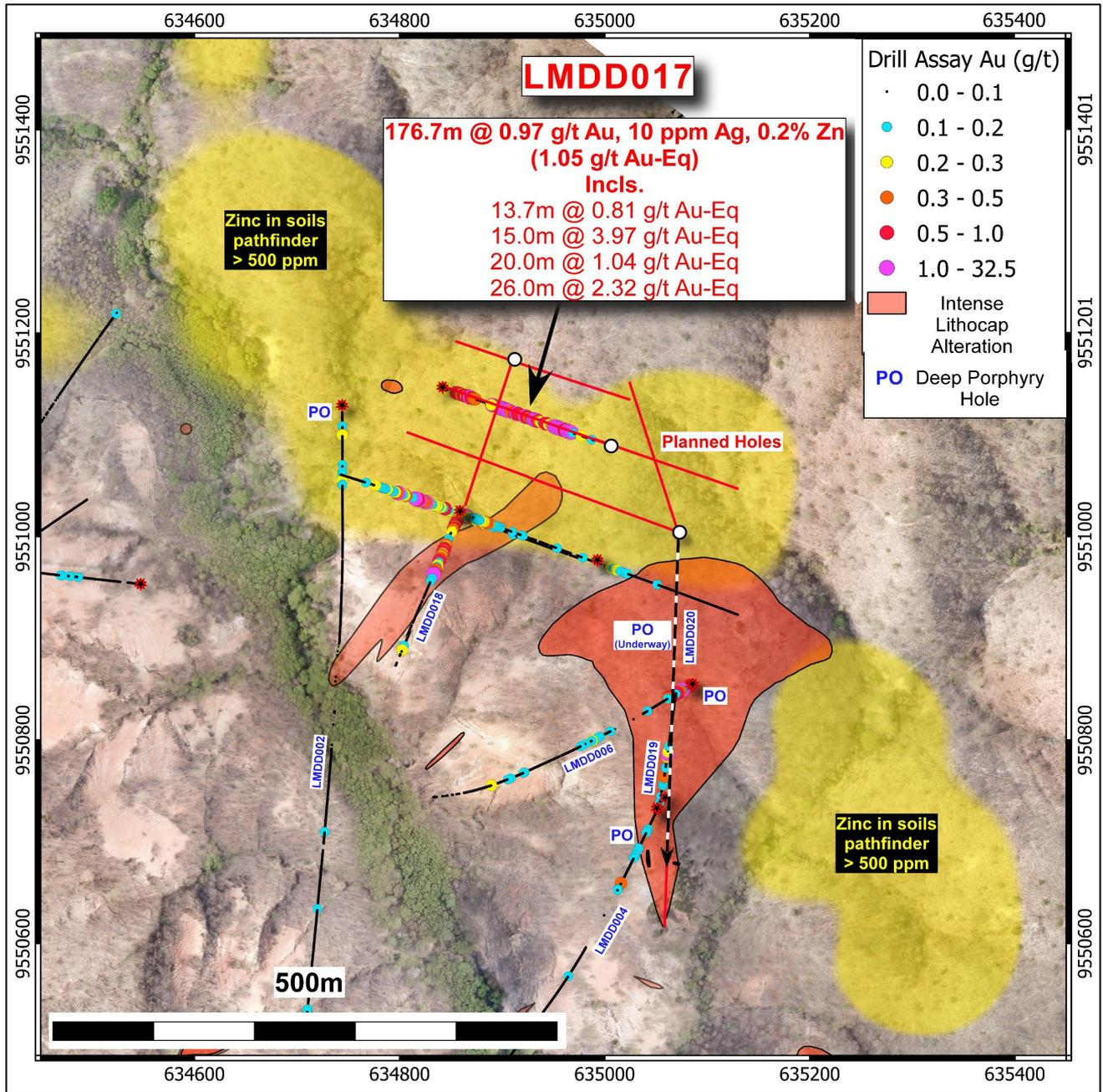
**Figure 3:** Area of epithermal mineralisation within the broader Limon target. Red lines show planned follow-up drilling to extend the multiple high-grade zones in LMDD017. Hole trace for LMDD020 is shown in the black and white dashed line, drilling from north to south at a dip of -66 degrees.
