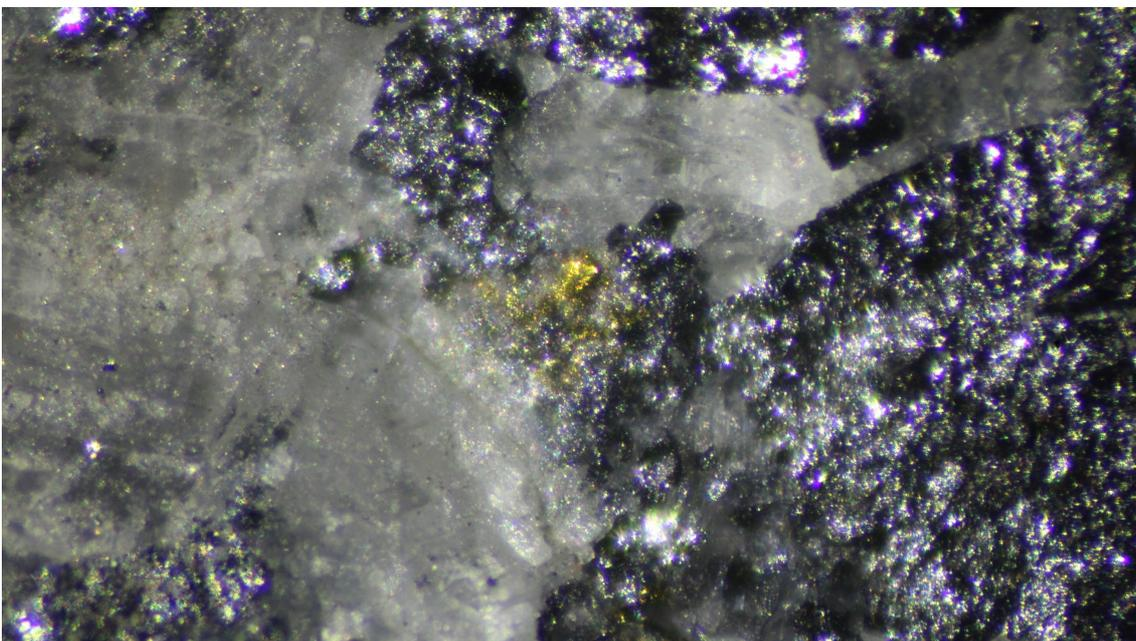
**Figure 2:** Photographs of visible gold and mineralisation style in LMDD020 at 665m down hole depth.
