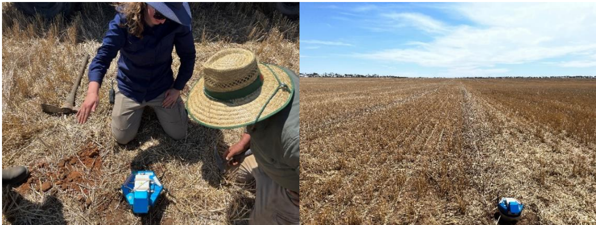
Photo Plate 1: Deploying sensors (Geodes) at Alford West, note the minimum surface disturbance.
