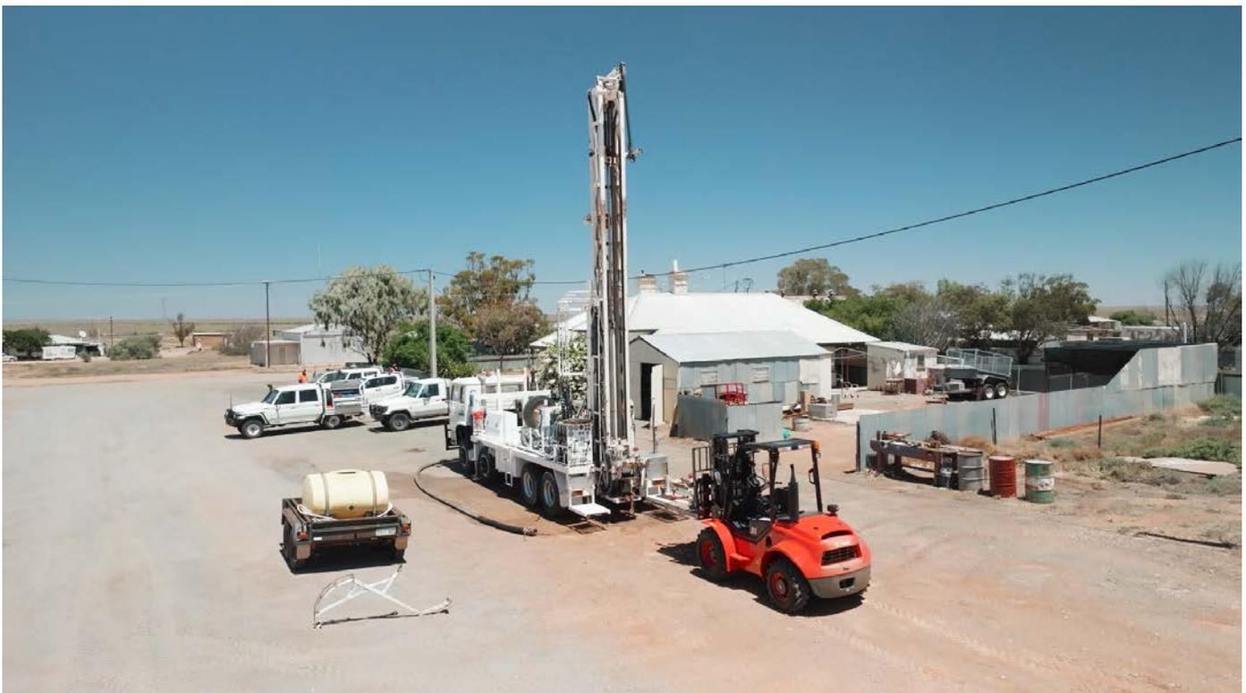
**Figure 2** Havilah's reverse circulation percussion drilling rig being serviced at Havilah's Cockburn exploration base-camp prior to being mobilised to the first of its planned 2023 drilling sites last week.
