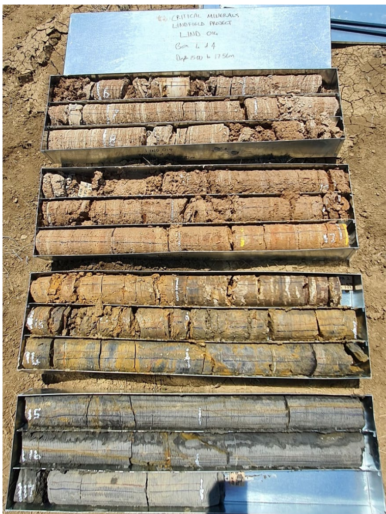
Image 3: Lindfield Project drill core from hole LIND014 showing the oxidised core intersection from 5.8m depth which contains both Vanadium and Alumina.
