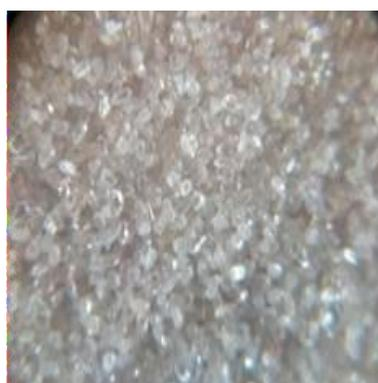
100x microscope image of Donald zircon grains. The zircon is seen as translucent white particles, with an absence of colour stains
