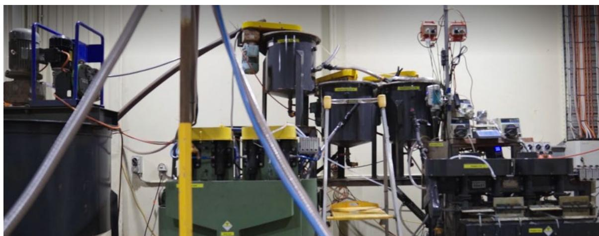
**Figure 18 – Continuous REE flotation pilot plant at Nagrom in Western Australia**
