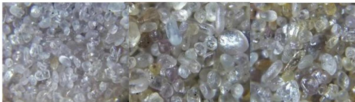
**Figure 48 – Competitor premium zircon grains under a 100x microscope**
