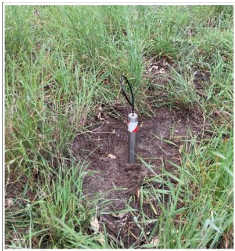
Figure 4 – Mid-term measurement via monitoring probe.
