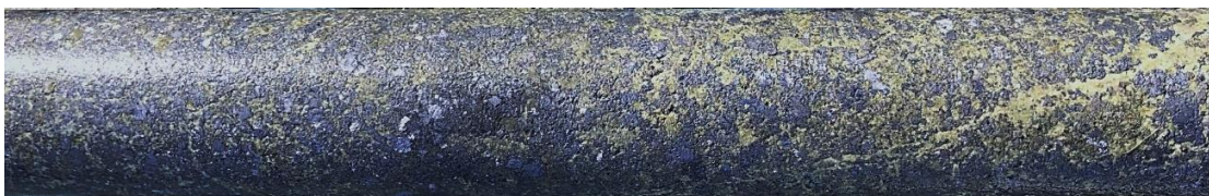
Image 1. Coarse blebs of galena (PbS) in core from drill hole WCS019
