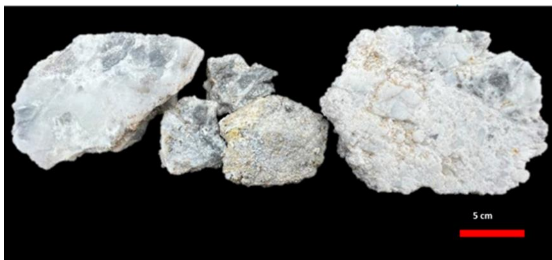
Figure 9: Samples of quartz vein from APD021. The quartz is crystalline and brecciated with clay-pyrite matrix. The section assayed 12.09g/t Au and 8.3 g/t Ag over 1m (42.2-43.2m)
