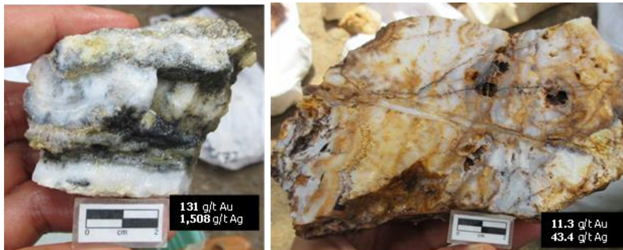
Figure 15: Photos of samples of vein material taken from artisanal miner pits. Refer to Figure one for sample locations. Both samples show the presence of crustiform banded quartz with thin dark-grey ginguro bands
