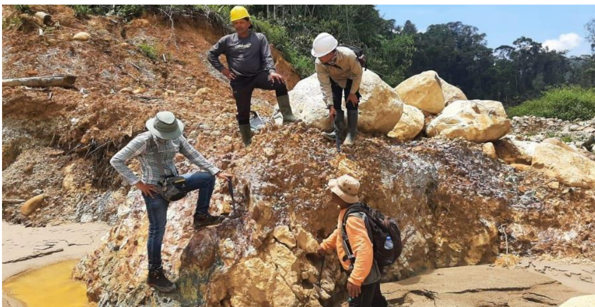
Figure 13: Above; Photos of rock grab samples of the Aloe Eumpeuk quartz veins taken from loose rock within artisanal mining pits. The samples shown contain multiple sites of visible gold and associated sulphides within massive, saccharoidal and vuggy oxidized quartz. Assays are pending for the samples. Below; photo of exposed quartz vein at Aloe Eumpeuk prospect.
