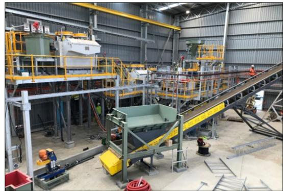
Figure 4 - View Inside Process Building looking east. With flotation area in the background and dryer feed conveyor in the foreground.
