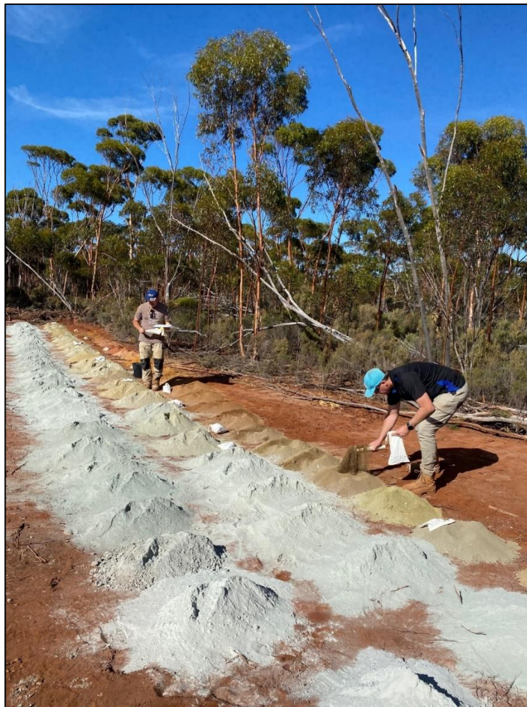
Figure 1 – Drill hole OLRC005 with pegmatite – Additional samples being collected specifically testing for nickel, cobalt and other base metals
