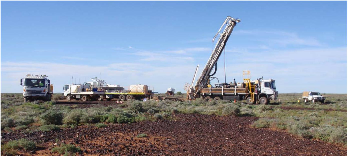
**Figure 4** Drilling copper anomalous gossan outcrop (dark brown ironstone scattered in the foreground) at the Johnson Dam prospect lying 14 km south-southwest of the Kalkaroo copper-gold-cobalt deposit.
