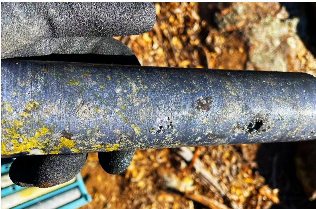
Image 1. Semi-massive Galena mineralisation in WCS050 drill core
