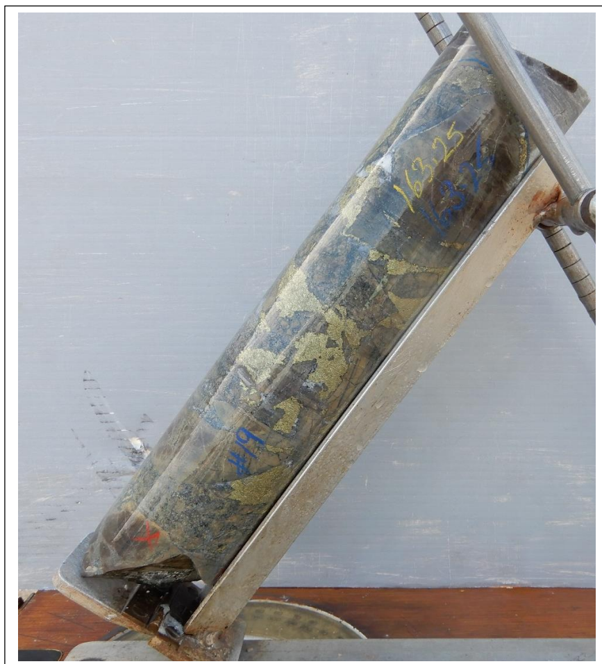
Fig. 4. Photo full HQ core Hole #19 , oriented in core oriented frame, hole drilling to south south west , view looking west north west , hole at 163.25m inclined at -44.5 degrees toward 206 degrees mag: Hydrothermal Infill Breccia. Clasts of light brown grey sericite altered hornfels, minor porphyry with infill of abundant chalcopryite (golden) , pyrite (brassy) ,minor calcite (white) ,quartz (glassy), dark green chlorite, fine rock flour.
