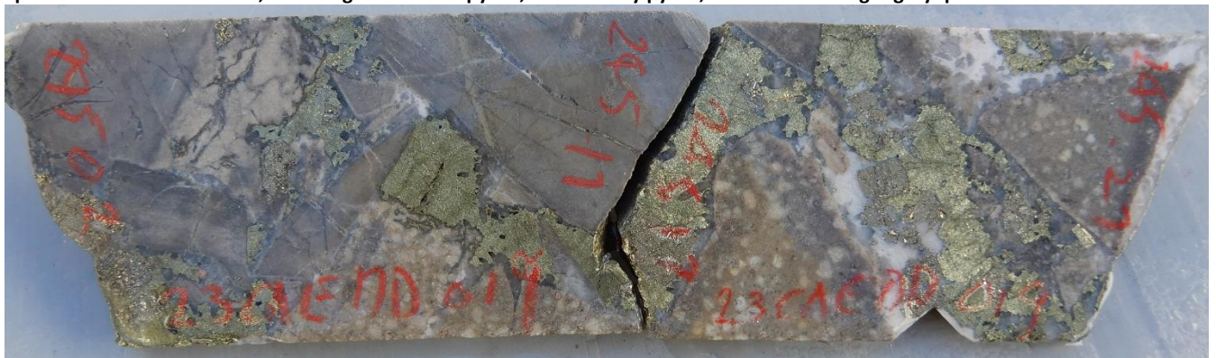
Fig 9. Photo Half HQ Core . Sulphidic hydrothermal breccia at 245m -. Angular clasts grey fine hornfels, feldspar porphyry, infill of golden chalcopyrite, brassy pyrite, white calcite & light grey well formed quartz.
