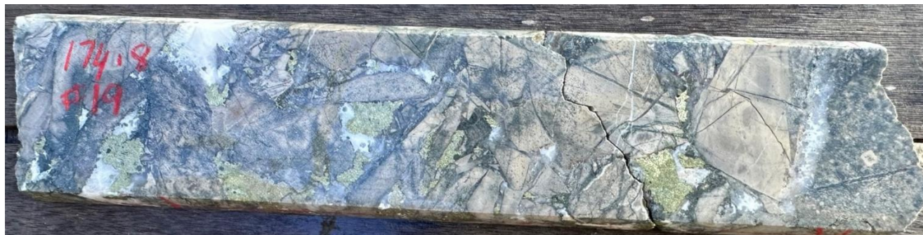
Sulphidic hydrothermal breccia at 174.8m -typical of interval 156m to 257m, CAE Hole 19 at Mt Cannindah. Drill to south south west between CAE Holes # 13 and 18, where CAE have recently announced high copper, gold and silver. Infill of golden chalcopyrite, some brassy pyrite, white calcite & light grey quartz. Angular clasts hornfels & some porphyry.
