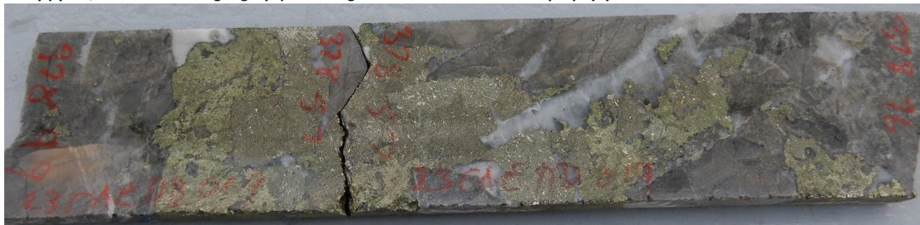
Infill in hydrothermal breccia of high grade chalcopyrite (golden) with well formed pyrite (brassy), some quartz (light grey) and calcite in a breccia dominated by angular clasts of yellow grey hornfels. CAE Hole 19, 378.5m intercepts.
