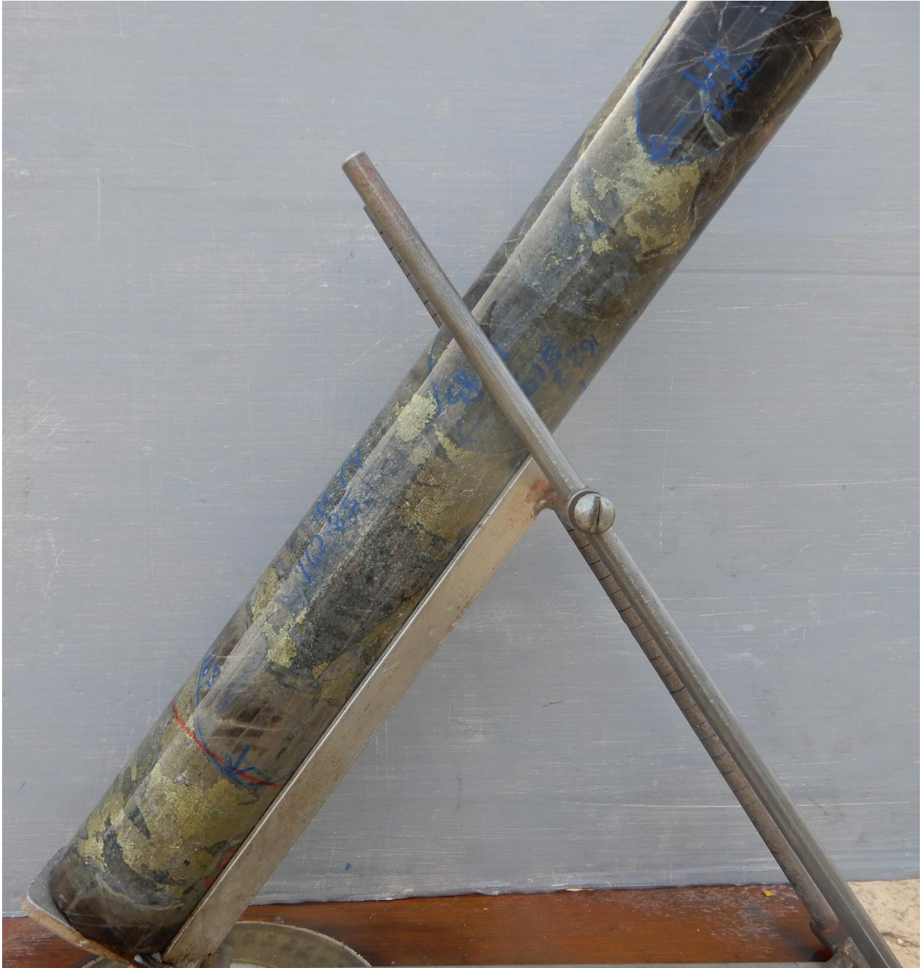
Fig 7. Photo - full HQ core Hole #19 , oriented in core oriented frame, hole drilling to south south west , view looking west north west , hole at 162.7m to 163m inclined at -53 degrees toward 217 degrees mag: Hydrothermal Infill Breccia. Clasts of grey, light brown grey hornfels, light grey where sericite altered, minor diorite porphyry clasts with infill of abundant chalcopyrite (golden) , pyrite (brassy) ,minor calcite (white) ,quartz (glassy), dark green chlorite, fine rock flour.
