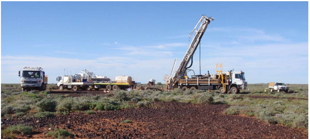
Figure 8 Drilling copper anomalous gossan* outcrop (dark brown ironstone scattered in the foreground) at the Johnson Dam prospect lying 14 km south-southwest of the Kalkaroo copper-gold-cobalt deposit.
