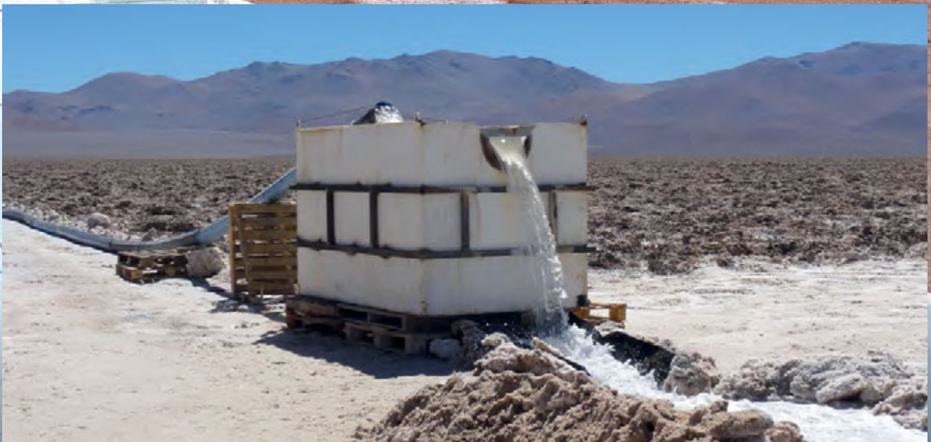
FIGURE 9: PUMP TEST AT MARICUNGA
