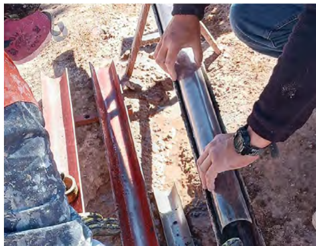
FIGURE 2: EXPLORATION DIAMOND CORE HOLES - DRILLING SAMPLES
