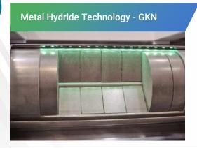
GKN Developed the first Commercial Solid State Storage System for Hydrogen with Integrated Electrolysers and Fuel Cells. The robust system generates green hydrogen from 100% renewable energy sources, storing it compactly and safely in metal hydride for reuse when there is no generation.
