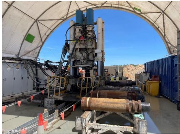
Figure 2: Raisebore Machine Excavating Ventilation Shaft
