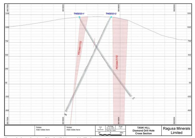
Figure 2. Cross Section of Tank Hill Diamond Drillholes
