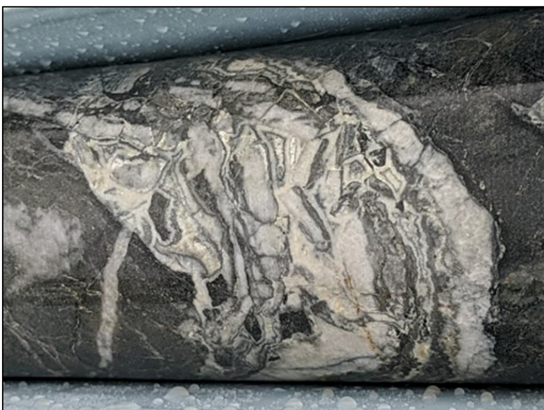
Figure 3: Left - 10cm wide crustiform qtz-adularia-sulphide vein breccia from 146m in PPDH182 drilled in 2022.
