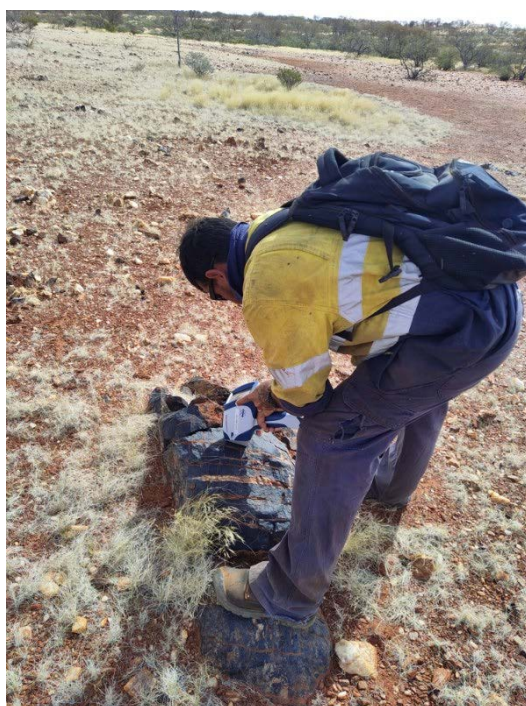
Figure 4 – Testing large tourmaline boulder with pXRF at newly discovered pegmatite outcrop.
