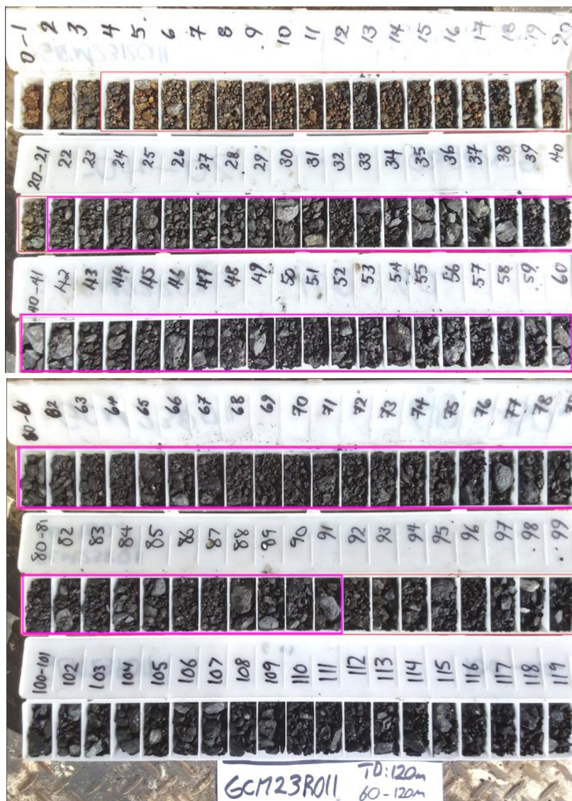
Figure 4 – RC chip samples from drillhole GCM23R011 showing visual graphite mineralisation. For estimates of abundance of graphite mineralization refer to Table 1 .
