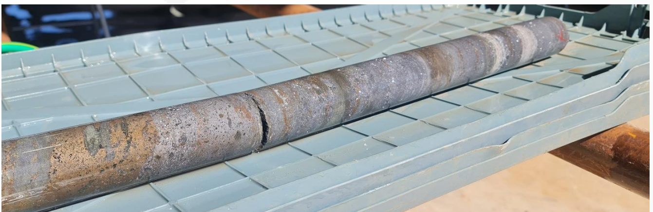
[Figure 1] MRN23008 - Core stick of semi-massive galena matrix breccia from the Western Horizon around 322m down hole.
