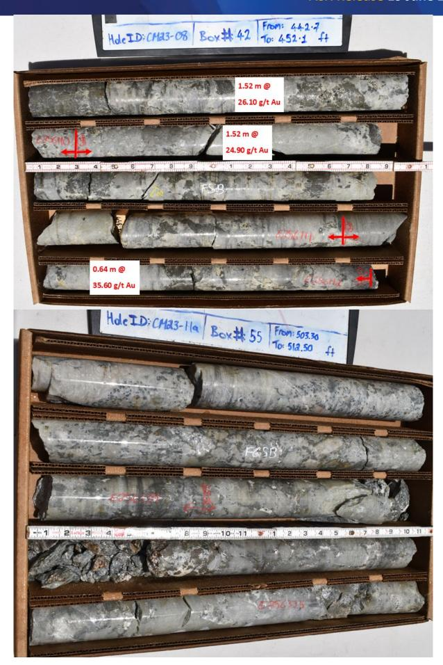
Figure 3: Photo comparing core from holes CM23-08 (top) to CM23-11a (bottom) demonstrating comparable core intersected in both drillholes
