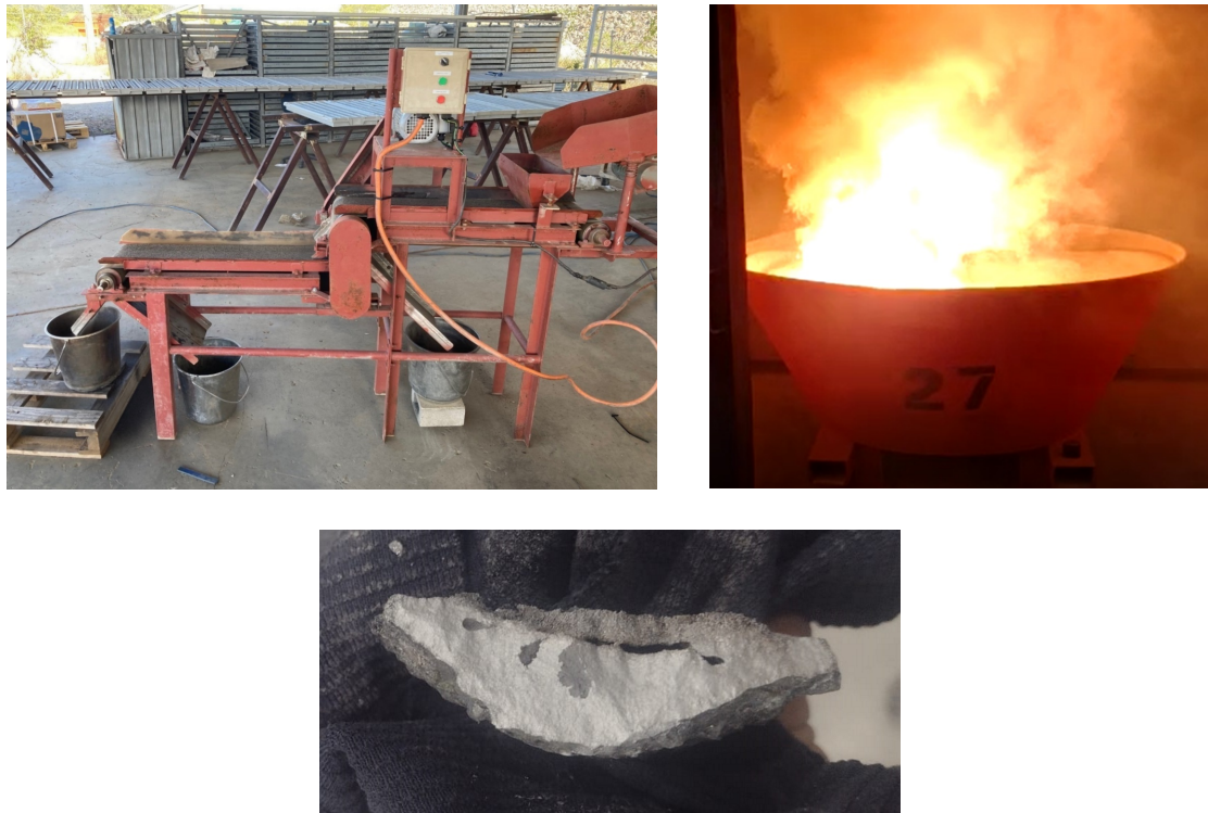
Fig. 2 - Top left: Pilot magnetic separator for separation of wolframite from scheelite concentrate; Top right: FeW smelting conversion testwork; Bottom: FeW sample from Mt Carbine (wolframite) concentrate
