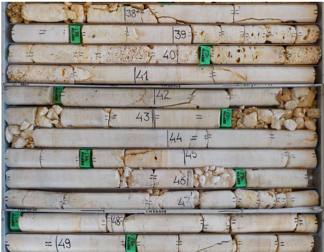
Fig 10 - VERY HIGH purity Limestone (CMDD008) from 37.88 to 49.53m, with weighted average 99.29% CaCO 3
