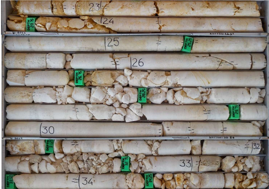
Fig 9 - VERY HIGH purity Limestone (CMDD006) from 23.02 to 34.70m, with weighted average 99.86% CaCO 3
