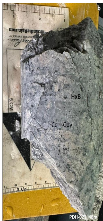
Figure 9 PDH-021 Hydrothermal breccia cemented by silica + secondary Chalcocite + Chalcopyrite, with clasts of dioritic porphyries. (6% sulphide)
