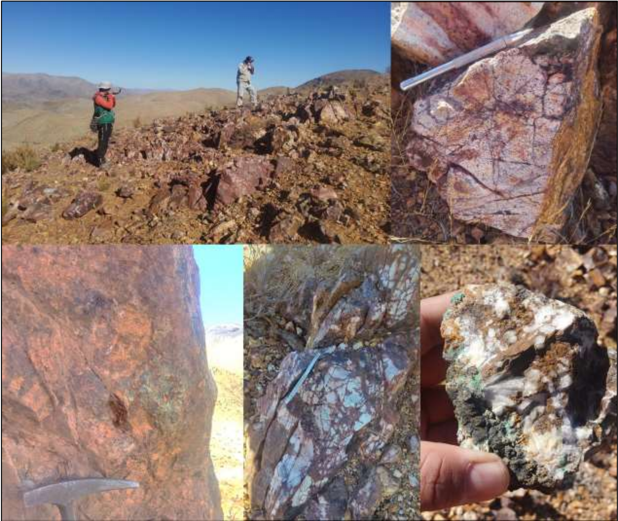
Figure 17. Photographs of stockwork veining and iron staining in the Venus 1 prospect. Intense stockwork of thin leached veinlets filled with quartz-goethite-red hematite-pyrite remnants. Chrysocolla (hydrous copper silicate) occasionally occurs filling the veinlets and fractures, however the rocks are largely leached. The swarm of veinlets has associated pervasive (100%) alteration of Sericite-Albite-Kaolinite-Silica-Smectite, in varying portions, mainly affecting the host volcanic sequence of the Cerrillos formation. The leached zone of stockwork contains boxworks (leached holes after pyrite and other minerals). Goethite is 10 to 15%, hematite approximately 5%, pyrite (boxworks y fresh) <2 %, and there are traces of secondary (non-sulphide) minerals.
