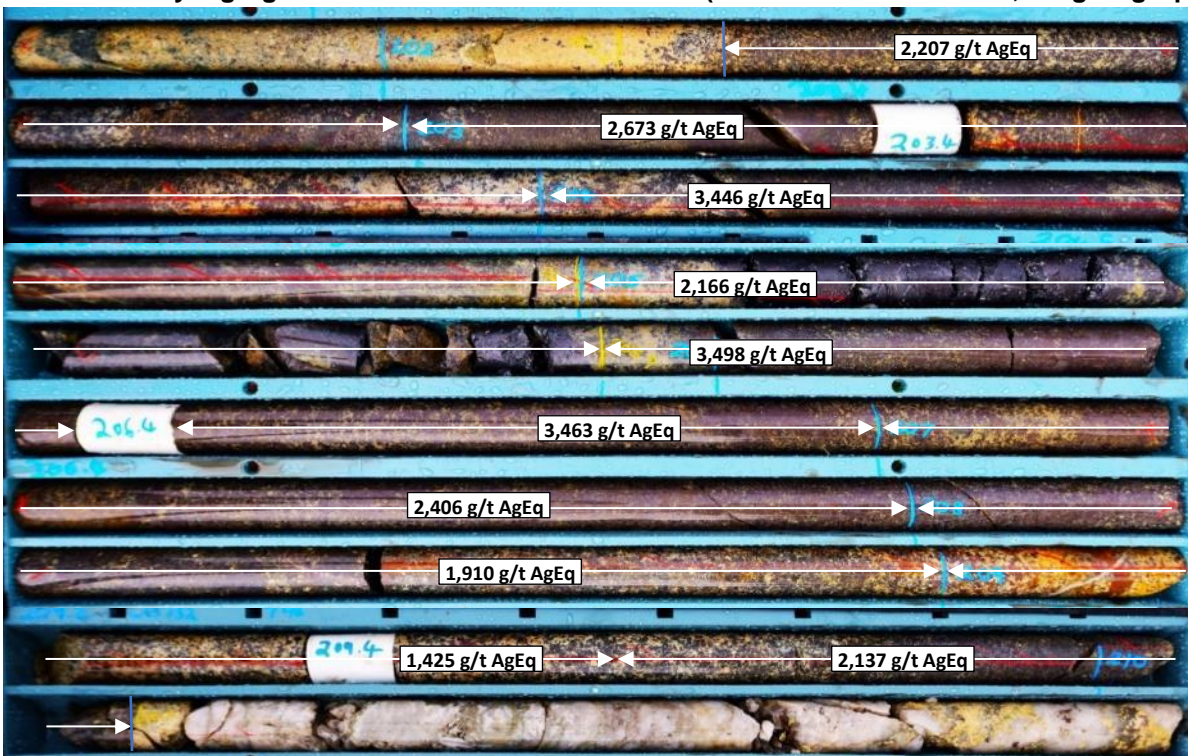
Photo 12. Very high-grade core from drill hole WCS052 (202.2-210.1m: 7.9m @ 2,519 g/t AgEq 1 )
