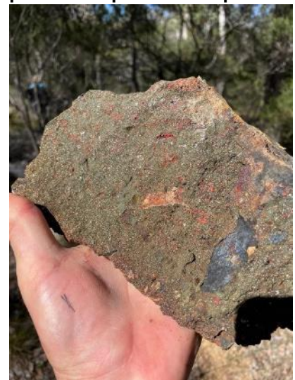
Photo 2. Strong chloritic alteration of leucogranite with pseudomorphs after sulphides
