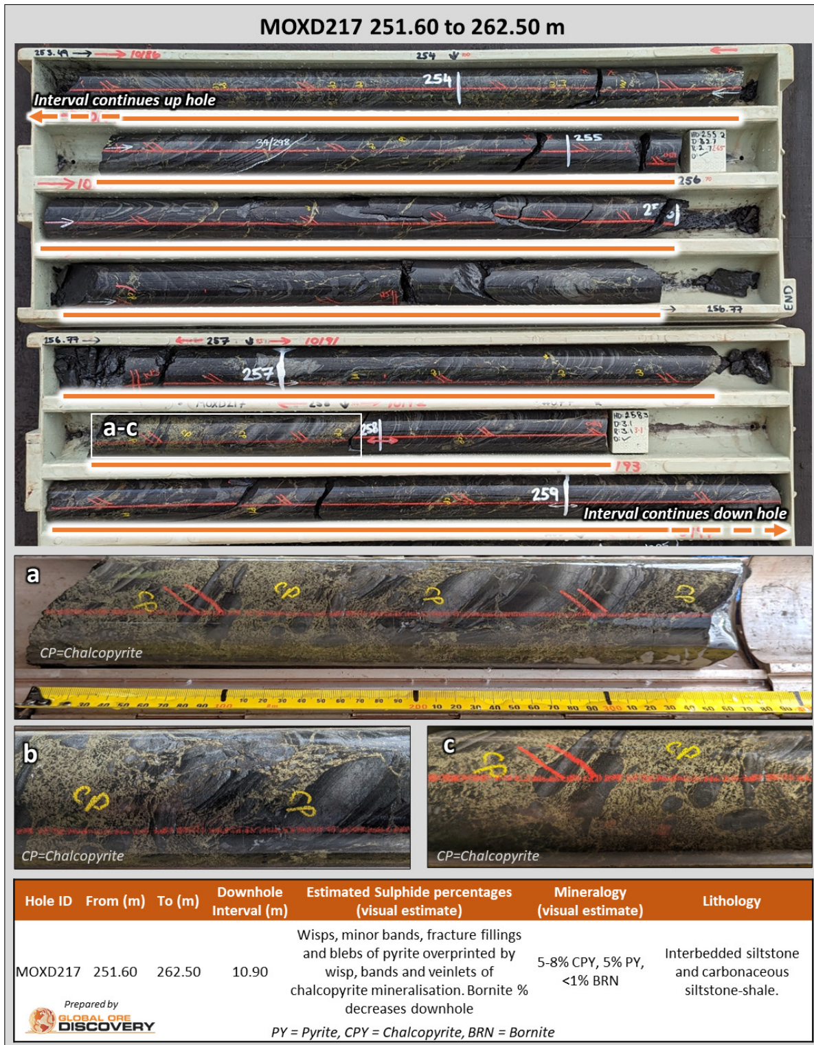
Figure 9 MOXD271 251.60-262.50 m 10.9 m wide zone containing wisps, minor bands, fracture fillings and blebs of pyrite overprinted by wispy, bands and veinlets of chalcopyrite mineralisation. Bornite percentage decreases downhole. (a) 257.60 - 257.96m strong chalcopyrite infill veining overprint pyrite infill of brecciated siltstone (b & c) MOXD217 – close ups of chalcopyrite infill veining in pyrite brecciated siltstone.
