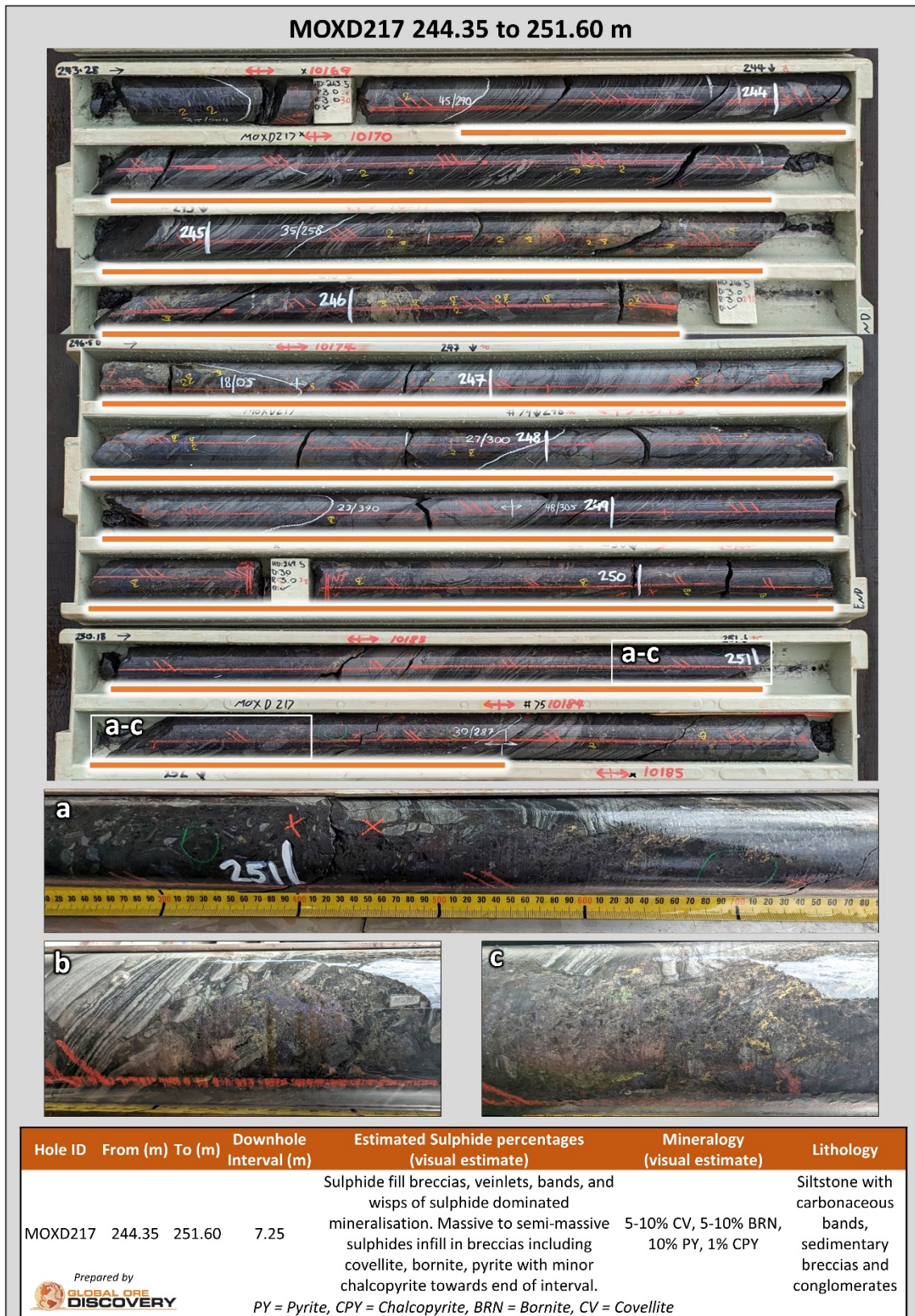
Figure 8 MOXD217 244.35-251.60 m- 7.25 m interval of sulphide fill breccias, veinlets, bands, and wisps of sulphide dominated mineralisation. (a) 249.82-251.38 brecciated siltstone with semi-massive sulphide fill. Sulphide fill includes covellite, bornite, pyrite, and minor chalcopyrite. (b & c) close ups of semi-massive sulphide fill breccias in siltstones.
