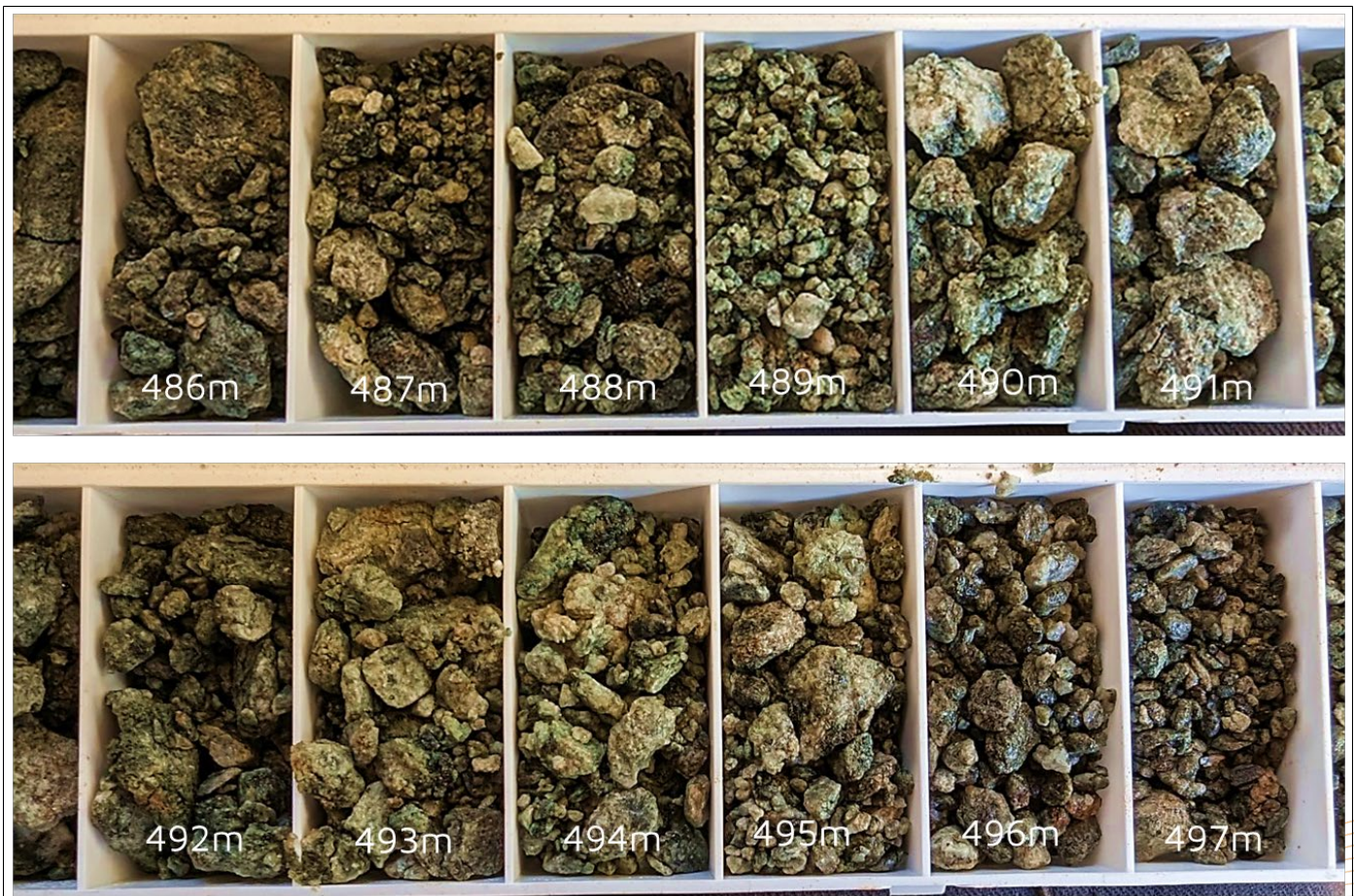
Figure 3. RC chips (486m to 497m) displaying a zone of intense biotite-actinolite altered komatiite with abundant quartz-carbonate alteration intersected from 474m to 497m (WDNRC002).
