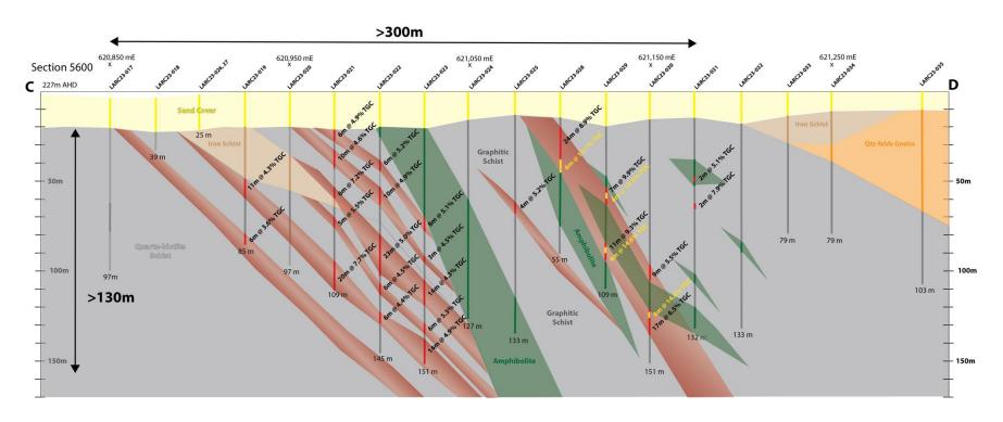
Figure 2. Traverse 2 - Section 5600, East-West section through the Lacroma Graphite Prospect – Scale 1:1
