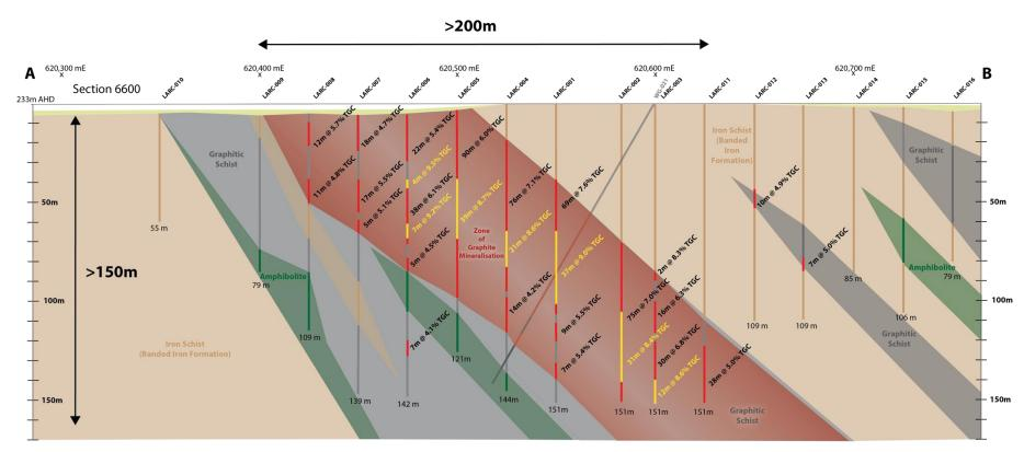
Figure 3. Traverse 1 - Section 6600, East-West section through the Lacroma Graphite Prospect - Scale 1:1
