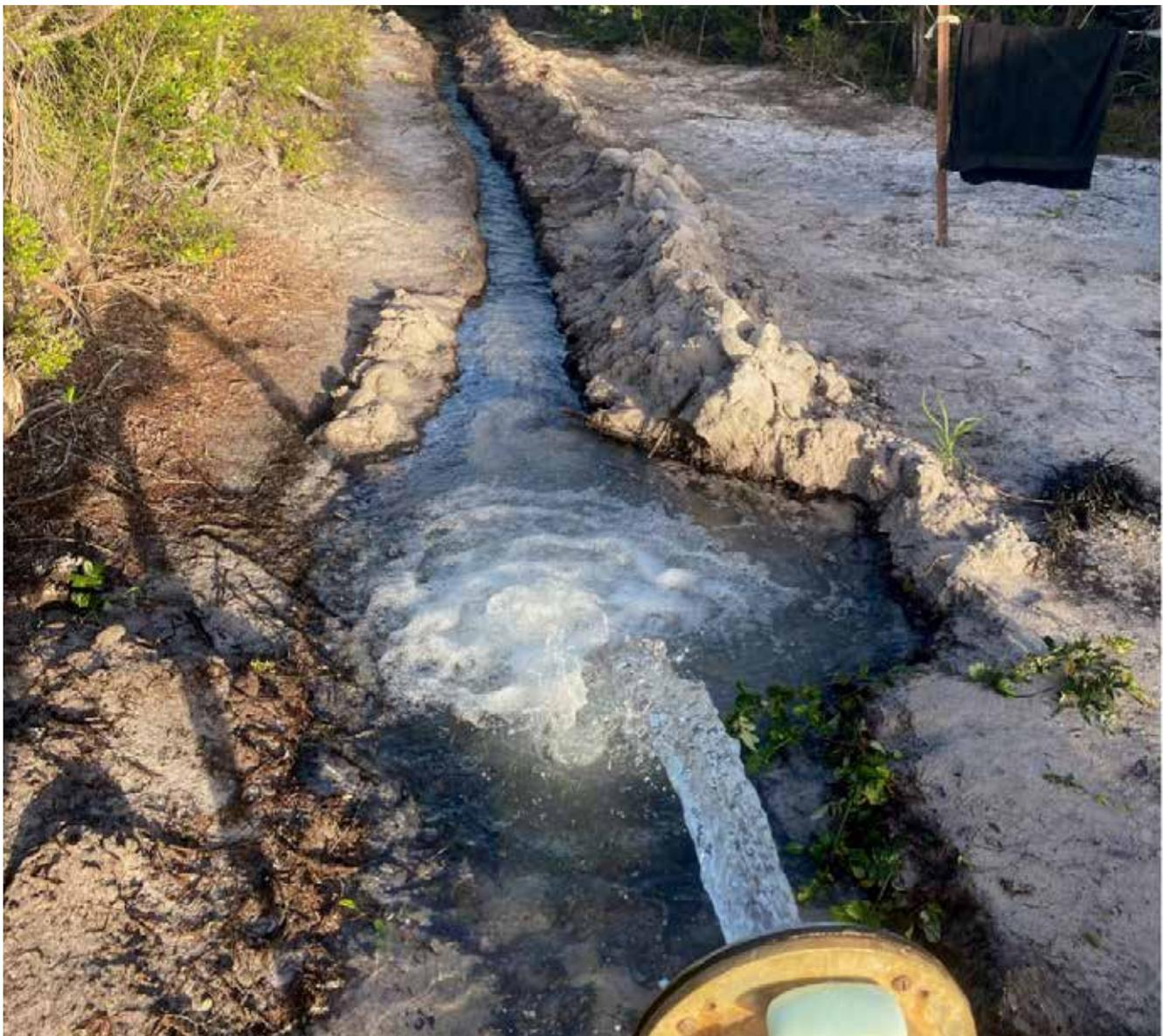
**Figure 4:** Water bore pump out test
