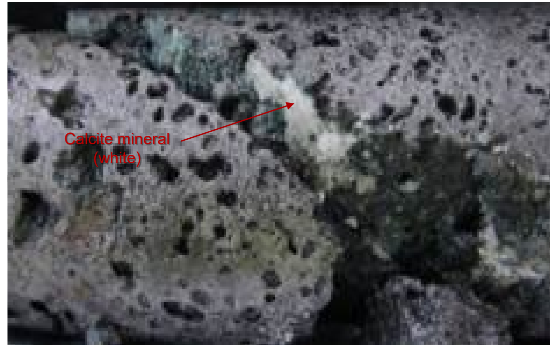
Image showing calcium carbonate (calcite) formed from CO 2 charged water injected into basalt at the Carbfix site in Hellisheioi, Iceland
