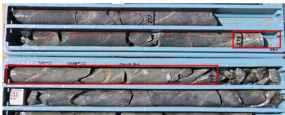
Figure 9: SP002 at 278-279m showing carbonate-quartz-sulphide veins with cream sericite and pink K-feldspar alteration selvage. This intercept assayed at 2.64g/t Au, 0.16g/t Ag, 0.023% Cu and 1,210ppm As
