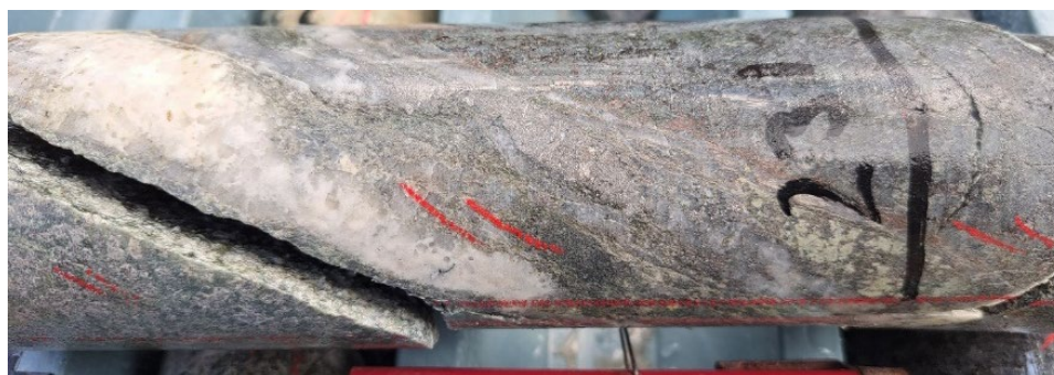
Figure 4: SP001 at 230-231m showing a carbonate-quartz-arsenopyrite vein. This interval assayed at 1.99g/t Au, 0.60g/t Ag, 0.024% Cu, >10,000ppm As
