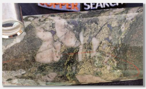
Figure 1. Quartz vein (15cm) with bornite (blue), pyrite and minor chalcopyrite at 221.2m
