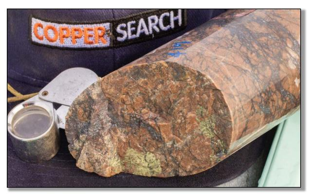
Figure 5. Face of HQ drill core at 419.7m – Hematite veins with chalcopyrite (brassy yellow)
