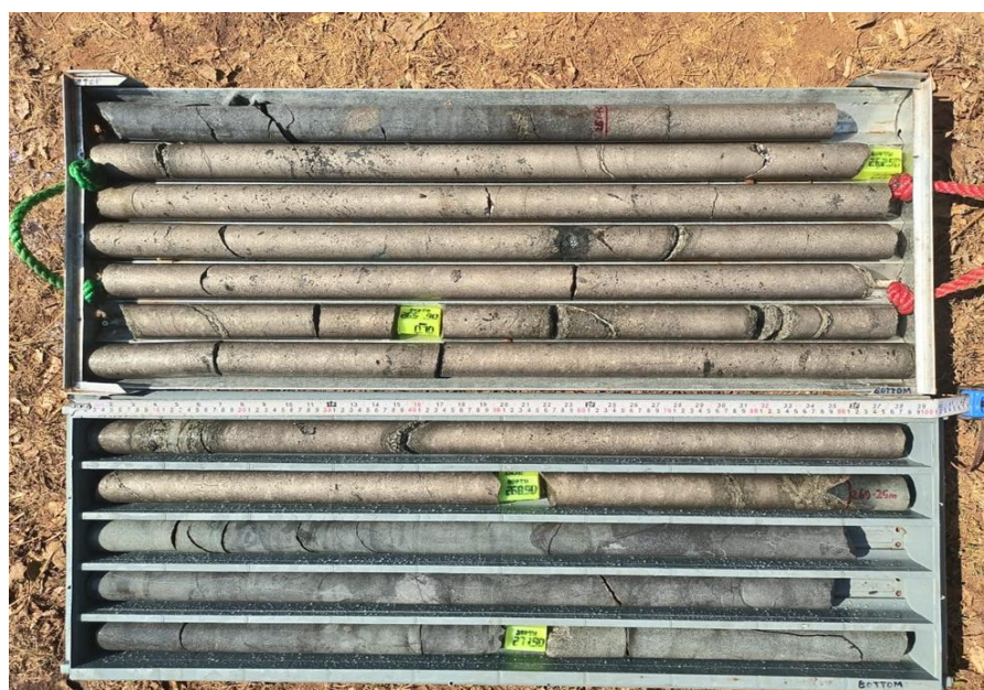
Figure 1 Photograph of 7.55m massive nickel sulphide intersection in DDLUHC003
