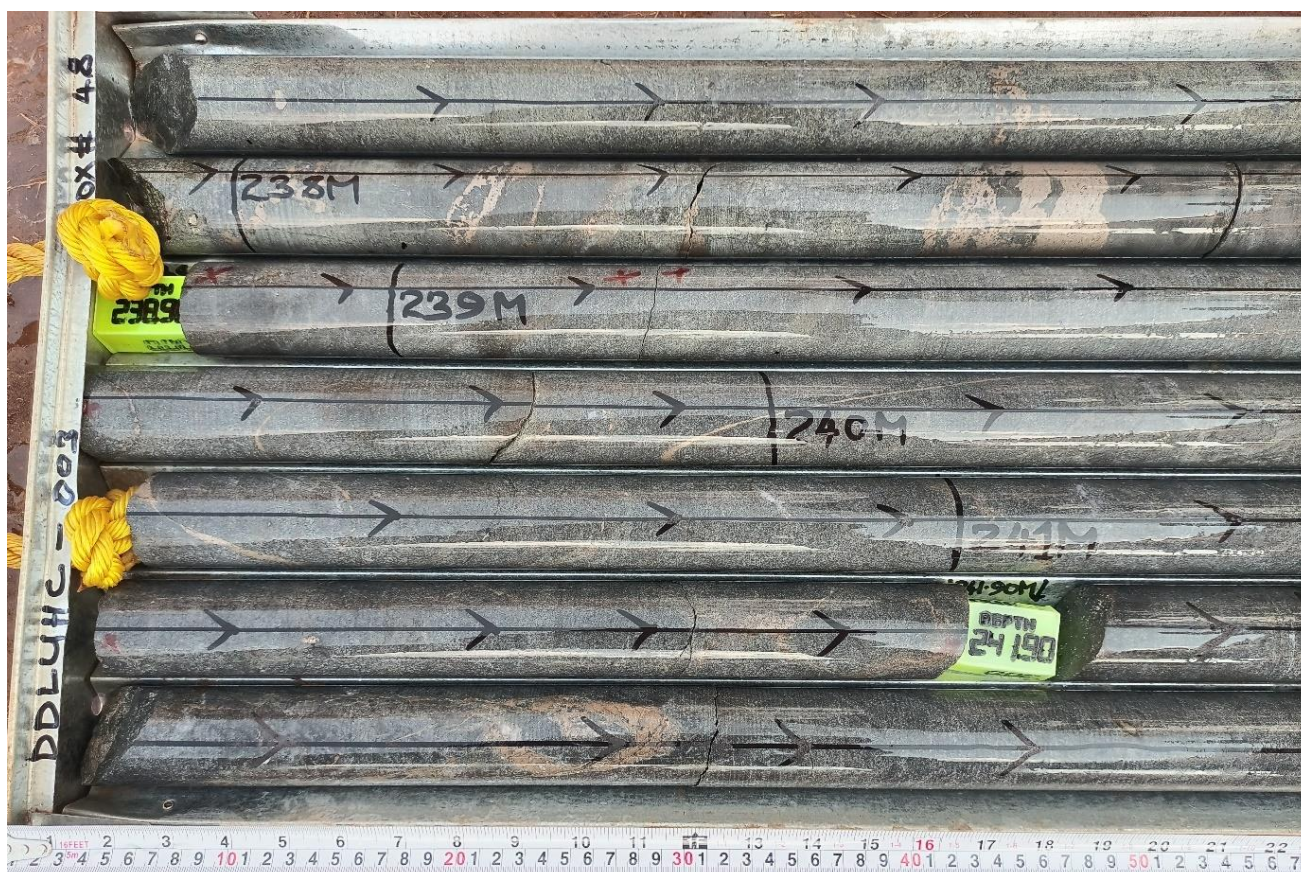
Figure 3 Photograph of 5.13m zone of thin semi-massive veinlets intersected in DDLUHC003
