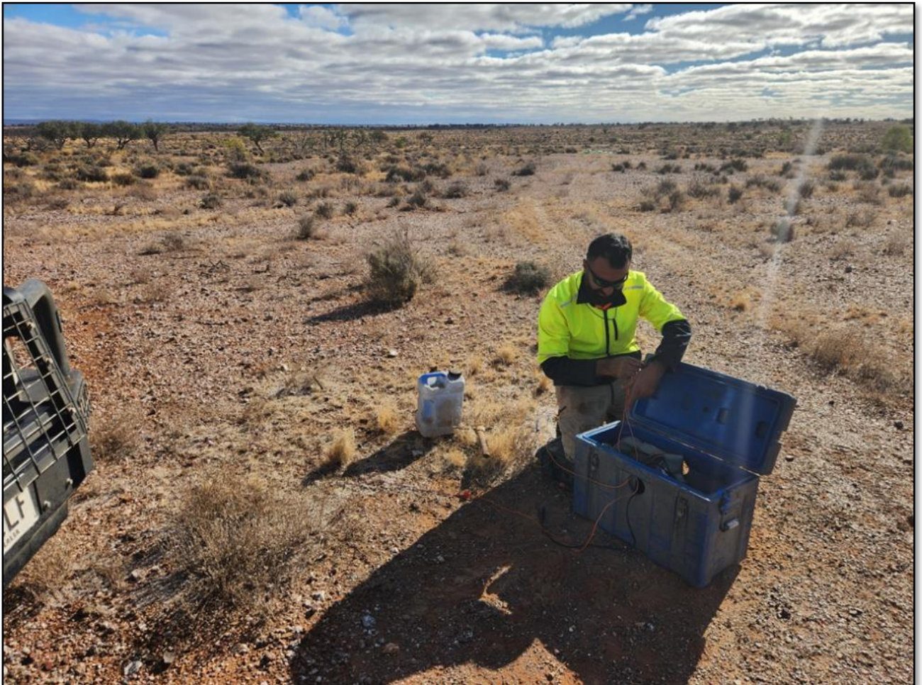
Figure 3 - CSAMT receiver station setup by Zonge geophysics
