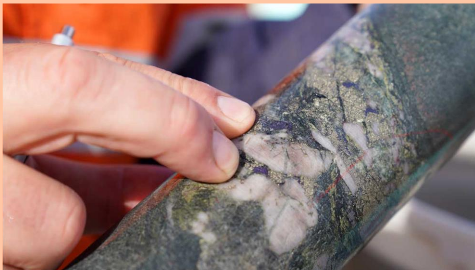
image: Quartz vein (15cm) with bornite (blue), pyrite and minor chalcopyrite at 221.2m
