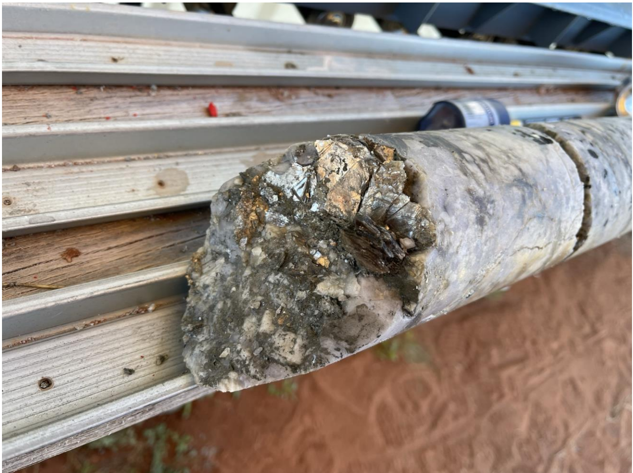
Figure 2: Sample core from diamond drilling during the quarter
