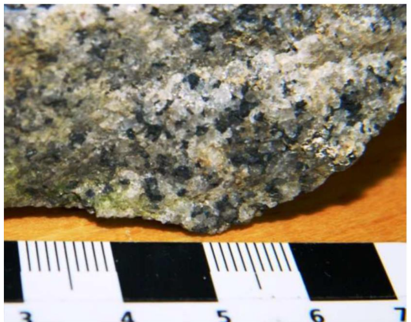
Figure 5 Silexite orebody with coarse grained tungsten mineralization (black crystals)
