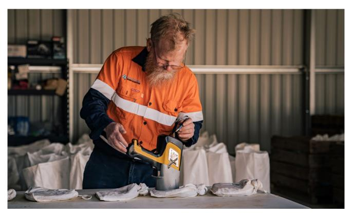
Picture - Samples being screened with XFR unit
